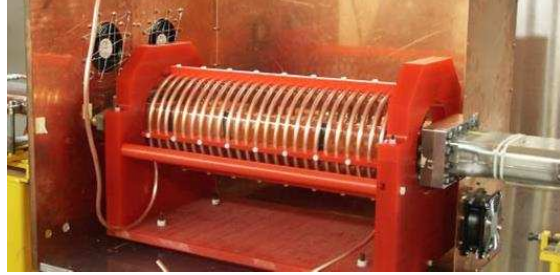
Figure 5.2: RF solenoid installed in the ring.
